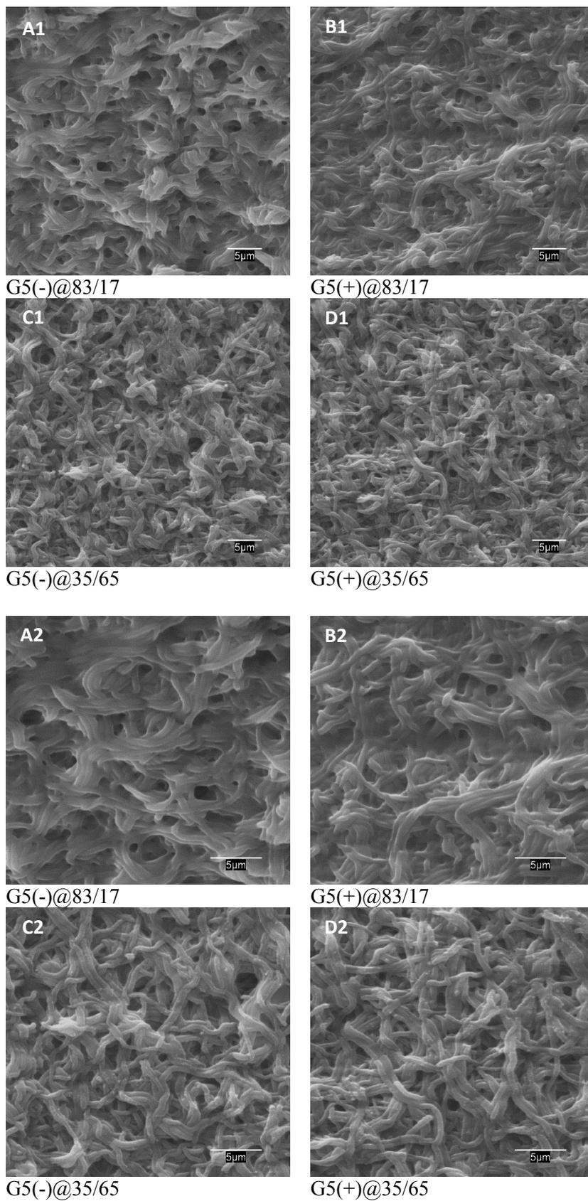
**Figure S2.** SEM images of PAMAM G5-NH<sub>2</sub>-functionalized membranes before (A1-D1) and after (A2-D2) thymol loading.
