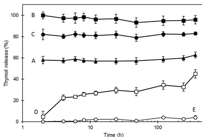
**Figure 3.** Release of thymol with the time in contact with different media: Water (A), acetic acid 30 g/L (B), ethanol 100 mL/L (C), ethanol 950 mL/L (D) and isooctane (E). The membrane, G5(+@35/65, was previously loaded with thymol as indicated in Table 3. Thymol concentration was recorded for 15 days, the later point representing 360 h.
