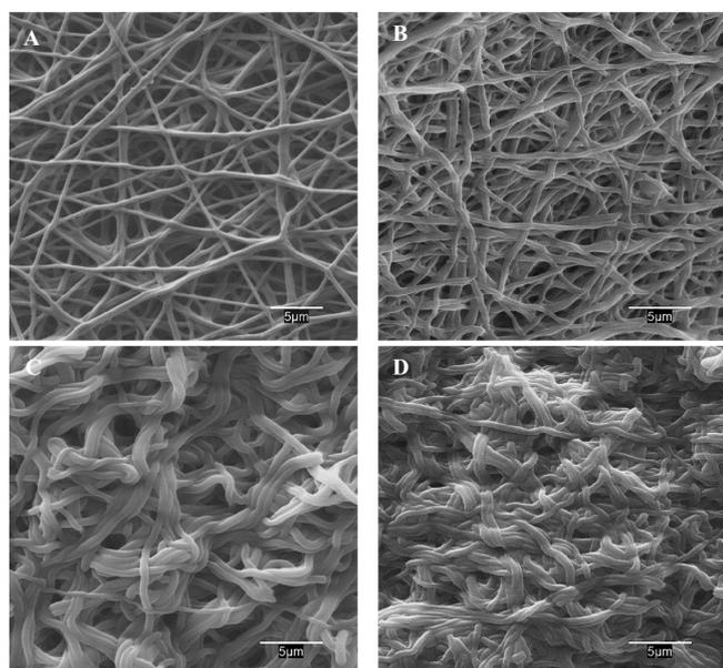
**Figure 2.** SEM images of PAA/PVA (83/17, A and 35/65, C) membranes and PAMAM G5-NH<sub>2</sub>-functionalized membranes G(+@83/17 (B) and G(+@35/65 (D).
