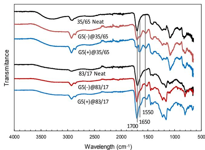
**Figure 1.** FTIR spectra of neat and PAMAM G5-NH<sub>2</sub>-functionalized membranes.
