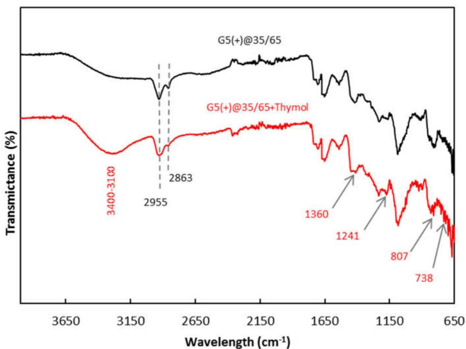
**Figure S1:** FTIR spectra of 35/65 PAMAM G5-NH<sub>2</sub>-functionalized membranes before and after thymol loading.
